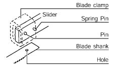
Fit the pin on the slider in the hole in the blade shank.
